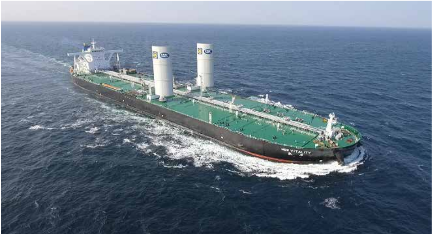
CMES' VLCC 'New Vitality' has been fitted with sails
